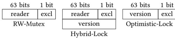
**Figure 2: Hybrid-Lock** – Combining optimistic and pessimistic
